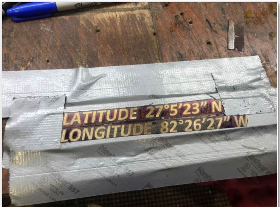
Acid etching brass strip with local lat/long using resist and duct tape.
